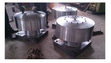
Thust Roller Assembly complete with Bearings
