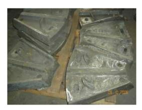
Ø3m x 10mL Cement Clinker Mill Feed Head Liner – Inner &Outer
