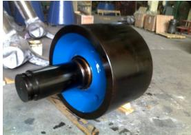
Forged Support Roller and Shaft Shrink-fitted as Assembly
